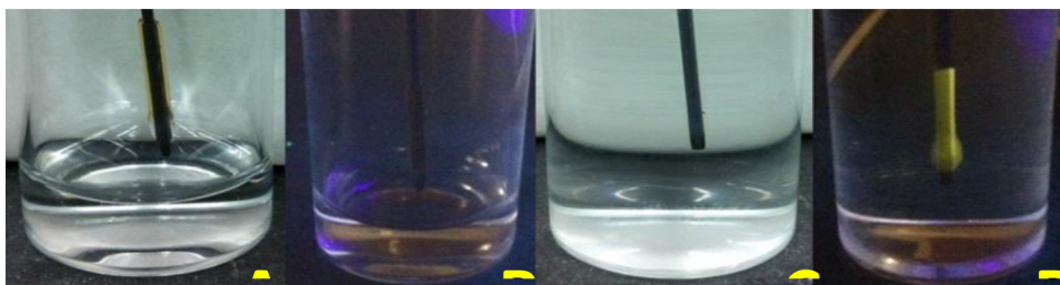
Fig. 5. Preparation of calcium cross-linked hydrogel coating through photoinduced reductive cation exchange of electrochemically deposited iron(III) cross-linked alginate hydrogel. (A) iron(III) cross-linked hydrogel deposited on graphite electrode at visible light; (B) the same under 254 nm UV light; (C) film of calcium alginate on the electrode after photochemical reduction, visible light; (D) the same under UV light.
